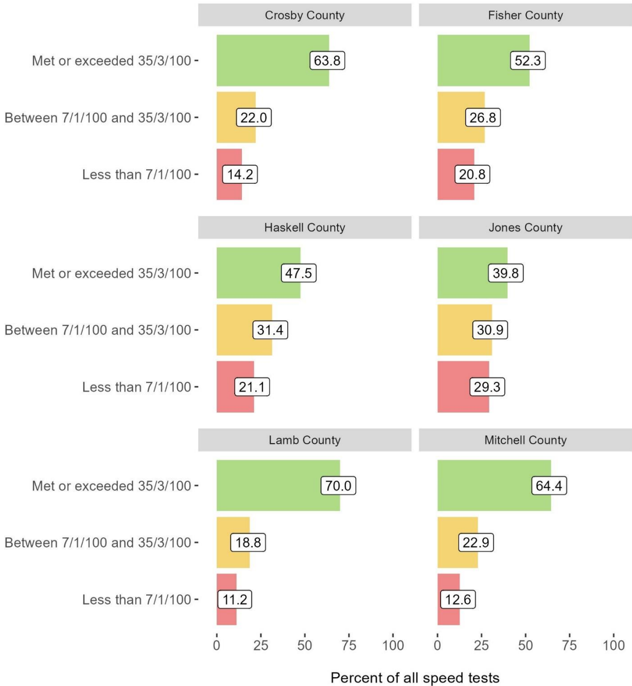
Figure 10. Percentage of mobile speed tests conducted in the 6 Texas TBP target counties by the Texas CLP team falling below the 7/1/100 threshold, falling between the 7/1/100 and 35/3/100 threshold, and meeting or exceeding the 35/3/100 threshold.
